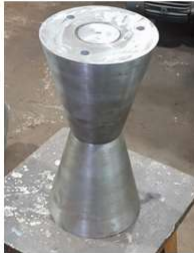
FIGURE 11: PICTURE OF ASSEMBLED PIN (THREADED BOLT) & CONICAL NUTS
